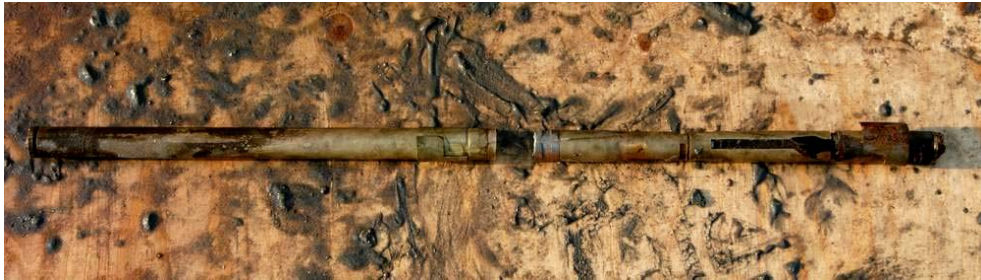
Fuse separated from the primer
